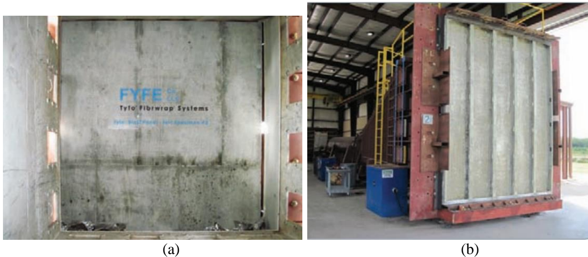
Figure 2.7 Blast Panels of Fyfe Co. in its tested specimen (a) interior, and (b) exterior [52]
