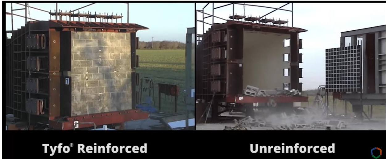
Figure 2.8 Blast Panels of Fyfe Co. in the conditions of two panels after explosive blast [52]
